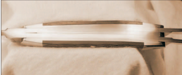
The whittler pattern uses a unique back spring design where the smaller blades each have their own spring but the main blade shares these two springs.
